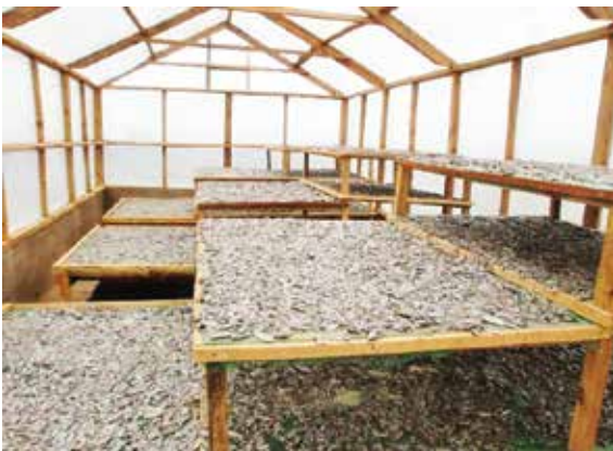
Plate 14 The initial pilot solar fish dryer was smaller (left) that was later enlarged and modified (right) following lessons learnt and increased demand from women fish processors from Kachulu beach, Lake Chilwa in Zomba. Photo credit: Welton Phalira and Precious Mwanza.
