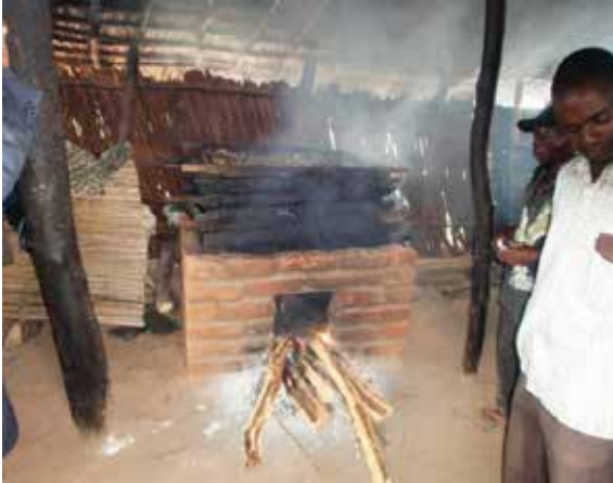
Plate 12 An open fish smoking kiln with several trays replaced the three stone open air kiln that used to smoke one fish tray at a time. Photo credit: Sosten Chiotha.
