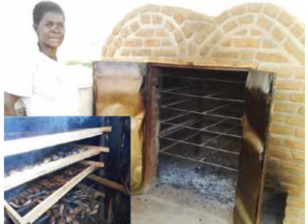
Plate 13 An improved fish smoking kiln with more and bigger trays in an enclosed chamber increases efficiency by confining the heat and smoke resulting in less firewood used. Photo credit: Joseph Nagoli.
